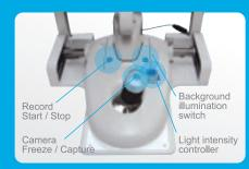
The Joy-stick features a shutter release, a video recording function, a background illumination switch and a light intensity control. Everything is on the unique shaped base of this slit lamp for ease of use. Still images and videos can be taken in one position.
